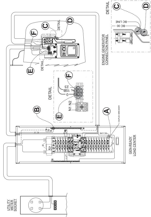
Figure 13. Test 46, 47, and 48 "GenReady Load Center" Test Points.
